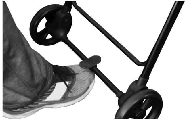
Brake is not applied when lever is up.
